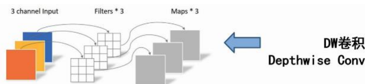
Figure 3. Schematic diagram of depth separable convolution feature extraction
