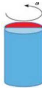
Fig. 2 Rotating permanent magnet type mechanical antenna
