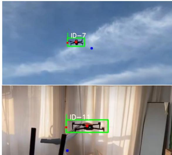
**Figure 21** UAV Recognition and Tracking Results
