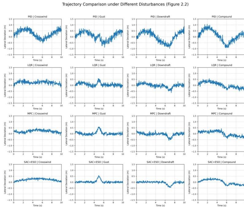
**Figure 2** Flight Trajectories under Different Disturbances. Rows: PID, LQR, MPC, SAC+ESO; Columns: Crosswind, Gust, Downdraft, Compound
