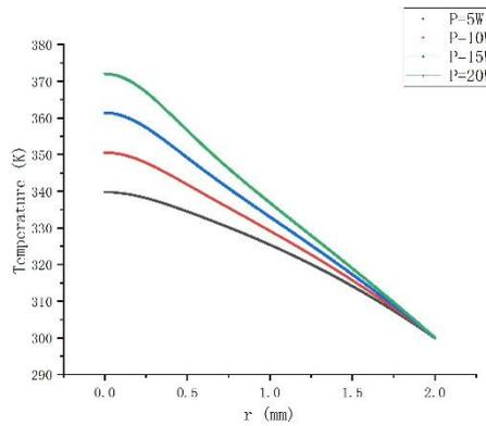
**Figure 6** Radial Temperature Distribution of the Laser Medium under Different Pump Powers
