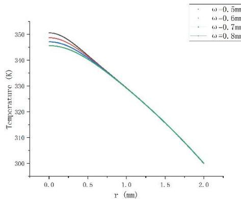
**Figure 8** Radial Temperature Distribution of the Laser Medium under Different Pump Beam Radii
