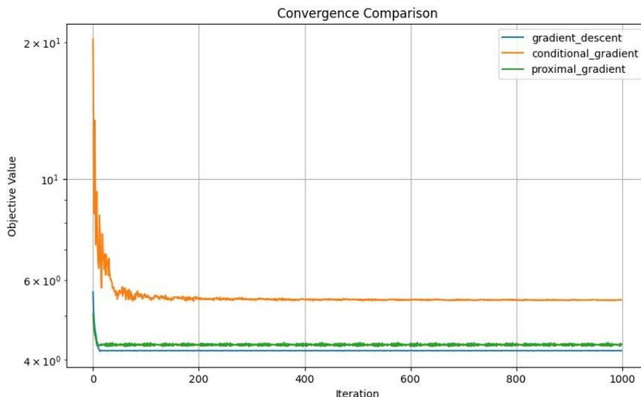
**Figure 1** Variation of Objective Values with Number of Iterations for Three Algorithms
