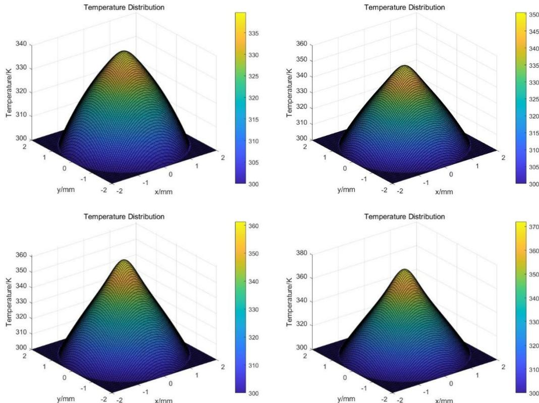
**Figure 1** Temperature Distribution at the End-Face of the Laser Medium under Different Pump Powers
