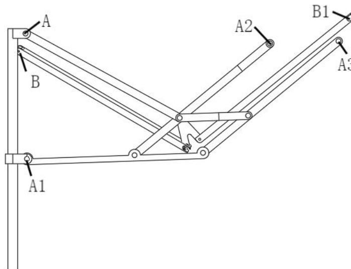
**Figure 1** Wing Extension and Retraction Mechanism
