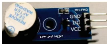
Figure 18 Physical Diagram of the Buzzer Module
