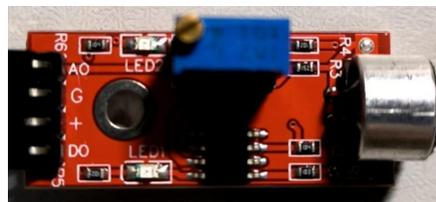
Figure 6 KY-037 Sound Sensor Module Physical Diagram
