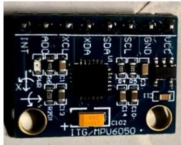
Figure 12 Physical Diagram of MPU6050 Gyroscope Module
