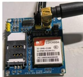
Figure 22 Physical Diagram of GSM Communication Module
