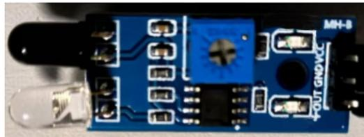
**Figure 8** Physical Diagram of Infrared Detection Module
