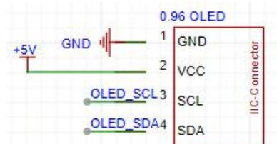
Figure 13 OLED Display Module Circuit Diagram
