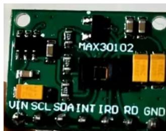
**Figure 10** Physical Diagram of MAX30102 Heart Rate Oximetry Sensor Module
