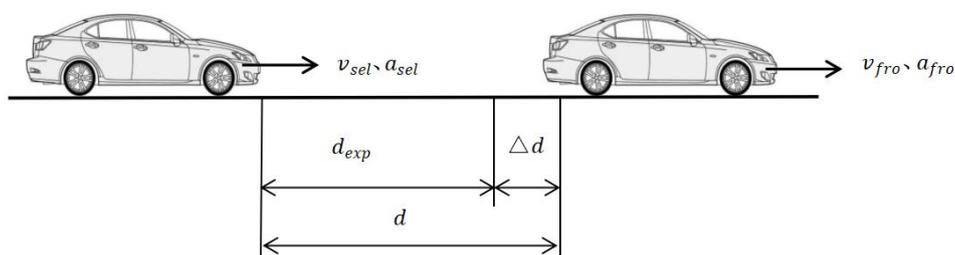
**Figure 3** Schematic Diagram of Vehicle Longitudinal Motion
