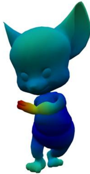
Figure 2 Visualization of Per-Vertex Deformation Energy (Blue: Low, Red: High)
