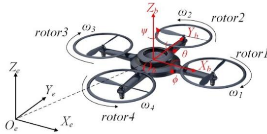
Figure 1 Coordinate Conversion and Rotor Structure of Four-Rotor UAV
